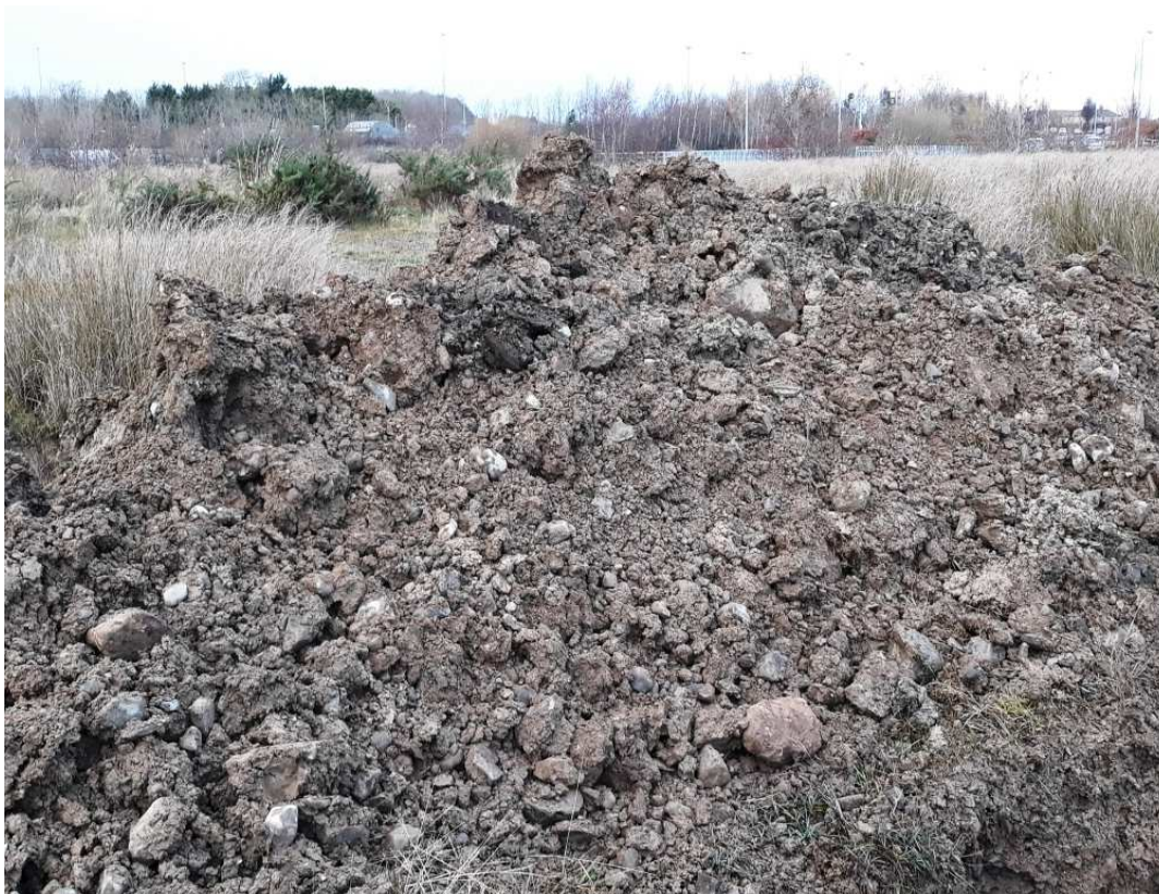
Figure 2 - Images showing MADE GROUND Deposits (Trial Pits 6, 7 and 11)
